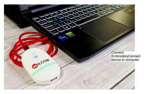
6 Ensure all lights are in 'Setup' mode as prompted. When the power LED is solid green and the WiFi LED is flashing blue, the device has finished booting. This generally takes about two (2) minutes.
