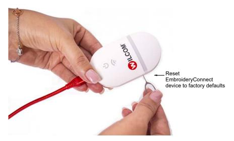
2 Hold for 10 seconds. This restores the device to whatever firmware it was initially programmed with. The EmbroideryConnect device can then be reconfigured using EmbroideryHub.
